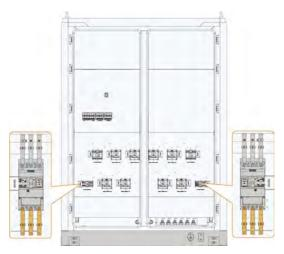
figure 5-12 AC power supply port
