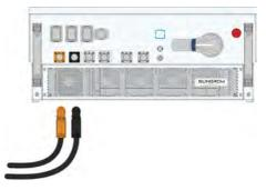
figure 6-3 Disconnect the power line between the Pack and the DCDC
