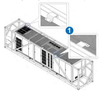
Step 1 Remove the corner fittings connecting the top of the BESS and the transport frame.
