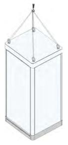
figure 4-7 Lifting diagram
