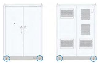
figure 4-11 Positions of L-shaped angle steels of LC1000
